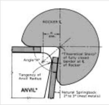
\*NOTE: The back taper relief ground on the anvil is to allow for the overbend required without pinching the material at full closure. (85° minimum anvil angle suggested for all 90° bends). Always grind 2° to 3° more back taper on anvil than the rocker's angle "A" being used.
